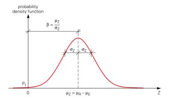
2.4 The reliability index  $\beta$  is a measure for the probability of failure.
